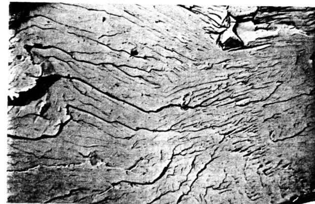
Fig. 5. River structure through ferrite in pearlite, replica \times 4,000 .
