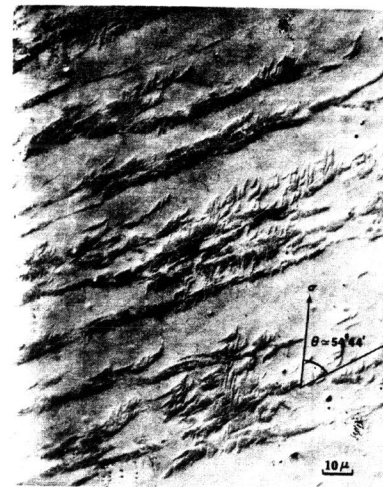
Fig. 8. Braggert martensite forming on tensile and shear axes of tensile specimen.
