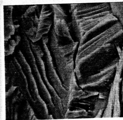
Fig. 2. Scanning electron micrograph of the fracture surface of a notched specimen of Ti-5Al-2.5Sn alloy pulled in 3% NaCl at a crosshead speed of 0.005 cm/min. (Magnification 430 x.)
