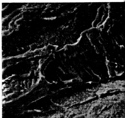
Fig. 6. Scanning electron micrograph of the fracture surface of a specimen of Ti-5Al-2.5Sn alloy cracked by charging in a solution of 0.03N H_2SO_4 at 50 mA/cm 2 for 14 days. (Magnification 710 \times .)
