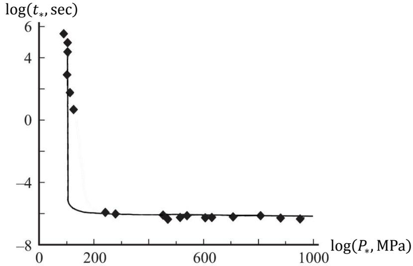
Fig. 1. Temporal dependence of strength for alluminium
