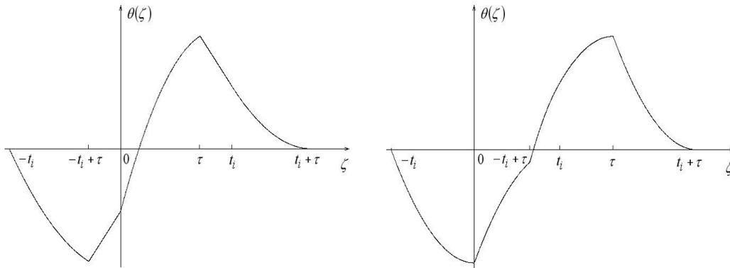
Fig. 2. Changing of damage function with time for long and short loading pulses.
