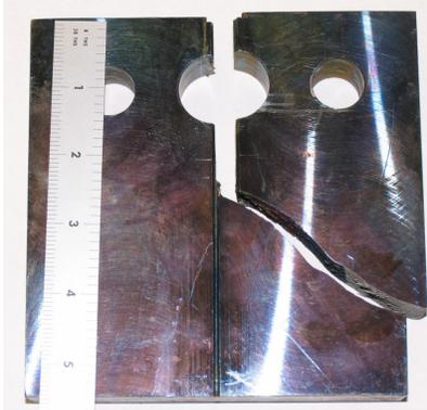
Figure 1 Compact crack arrest specimen with crack growing out of intended crack plane.
