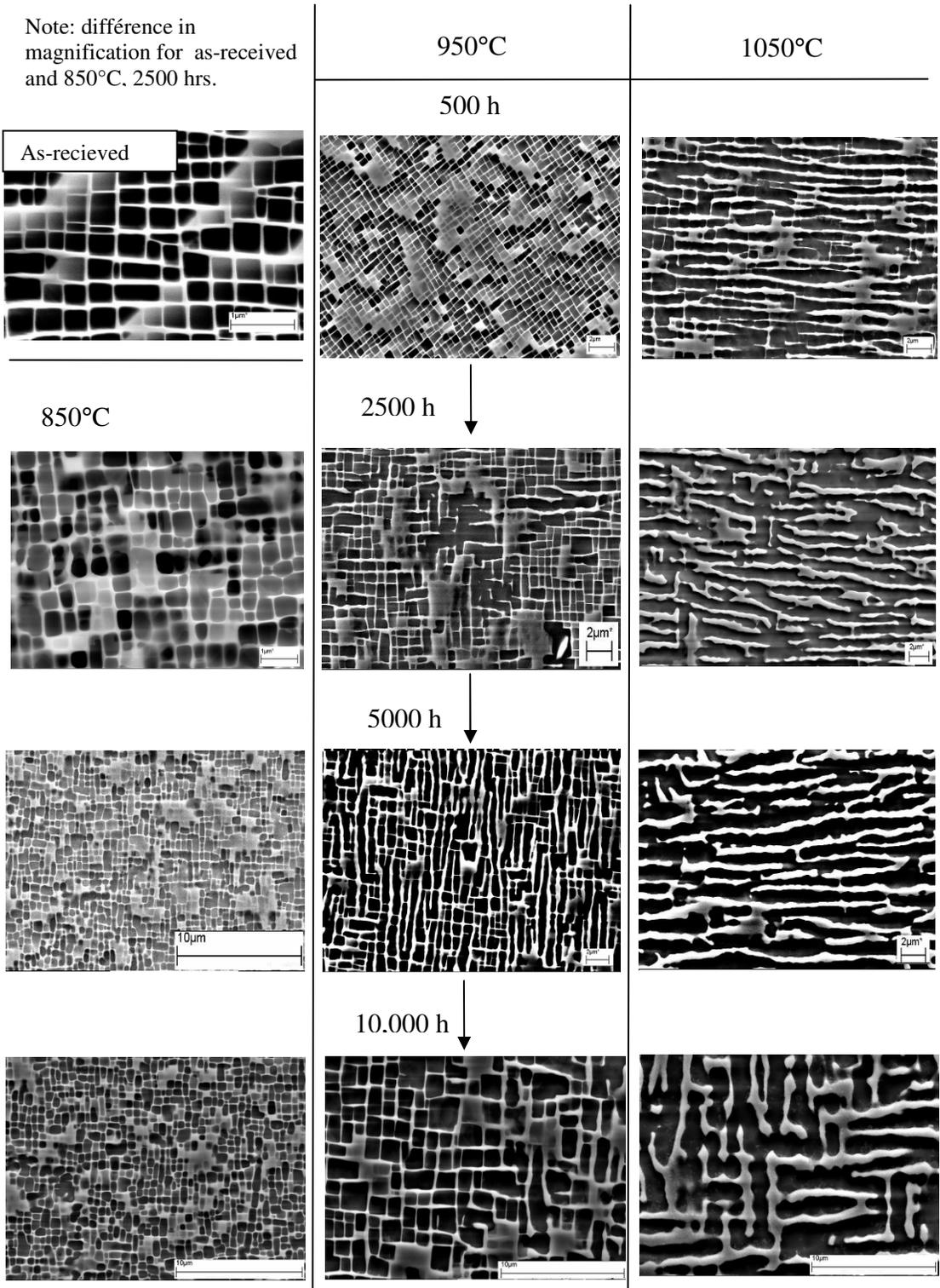
Figure 1 FEG-SEM images of thermally exposed CMSX4 at 850, 950 and 1050°C. All images are of approximately equal magnification, except where stated.
