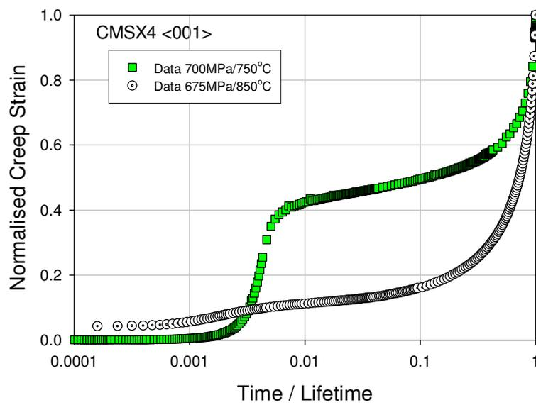
Figure 3 Creep response of CMSX4 showing very different shapes of creep curve.
