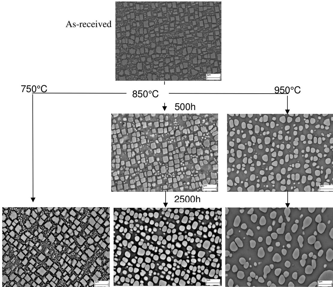
Figure 2 FEG-SEM images of thermally exposed IN738LC samples at 750, 850 and 950°C.
