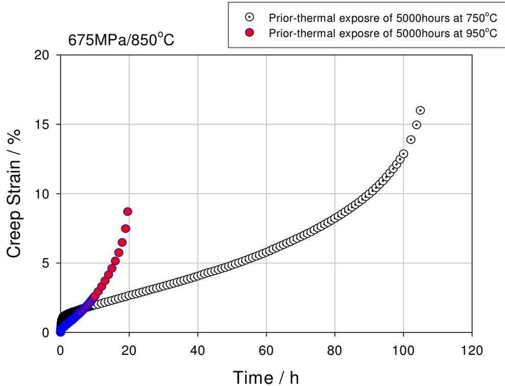
Figure 4 CMSX4 <001> creep response at 675MPa/850°C after 5000 hours thermal exposure at 750 and 950°C.
