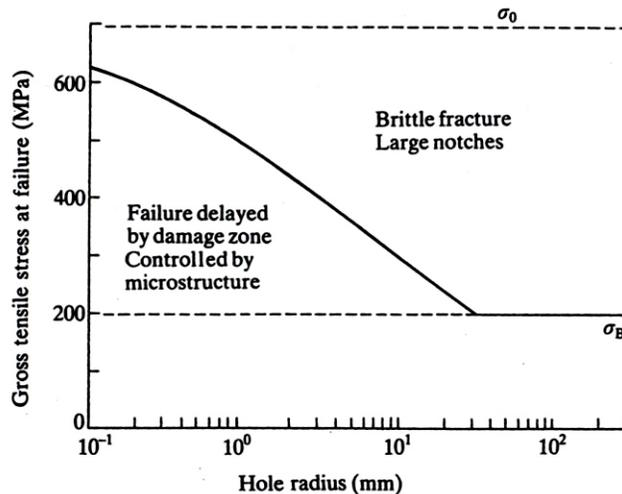
Figure 1 shows schematically the effect of holes on the strength of carbon fibre-reinforced epoxy laminate according to these ideas.
