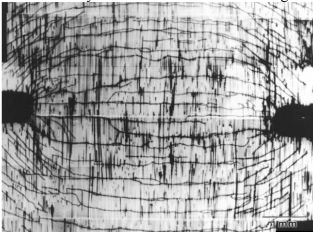
Fig 3. Cracking in a notched specimen of 40% SiC fibres in a calcium aluminosilicate glass.
