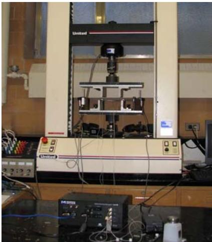
Fig. 12 4-point bend test system showing that the FBG strain sensing unit (the black box) connected with test sample with optical fibers .
