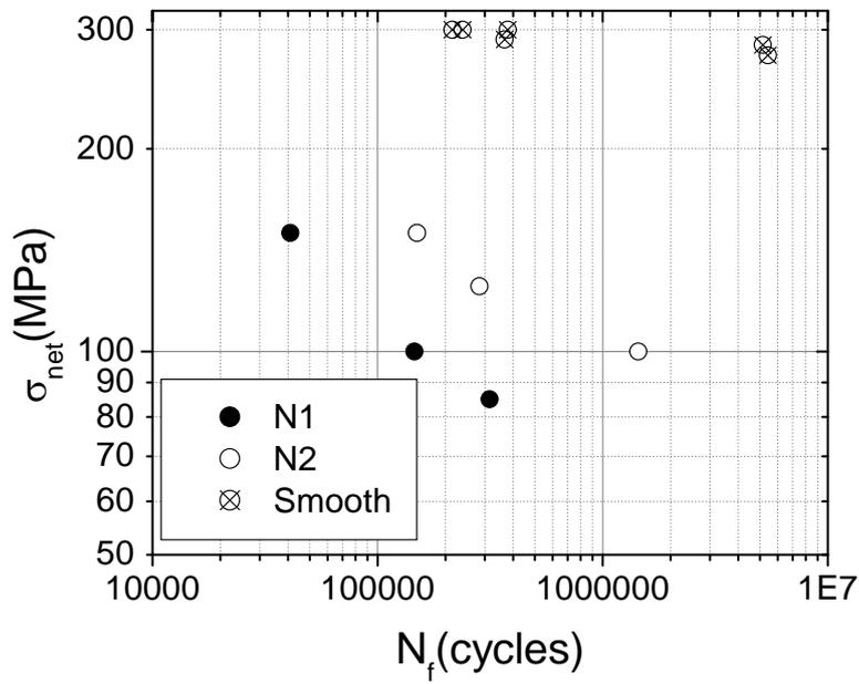
**Figure 2 :** Total fatigue lives plotted against nominal stress amplitude for notched specimens and smooth tubular specimens under axial loading.
