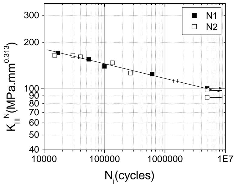
**Figure 5 :** Macroscopic crack initiation lives of notched specimens N1 and N2 under torsional loading against the amplitude of mode III notch stress intensity factor.
