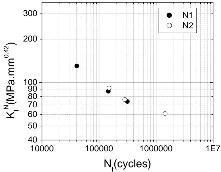
**Figure 4 :** Total fatigue lives of notched specimens N1 and N2 under axial loading against the amplitude of mode I notch stress intensity factor.
