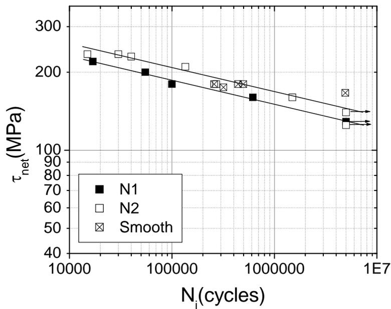
**Figure 3 :** Macroscopic crack initiation lives plotted against nominal stress amplitude for notched specimens and smooth tubular specimens under torsional loading.
