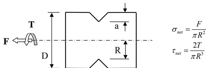
**Figure 1.** Schema of specimen central part and definition of nominal stresses over the net section (F = axial load; T = torque)
