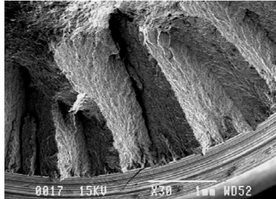
**Figure 6 :** Factory-roof fracture surface observed all around specimen circumference under cyclic torsion.
