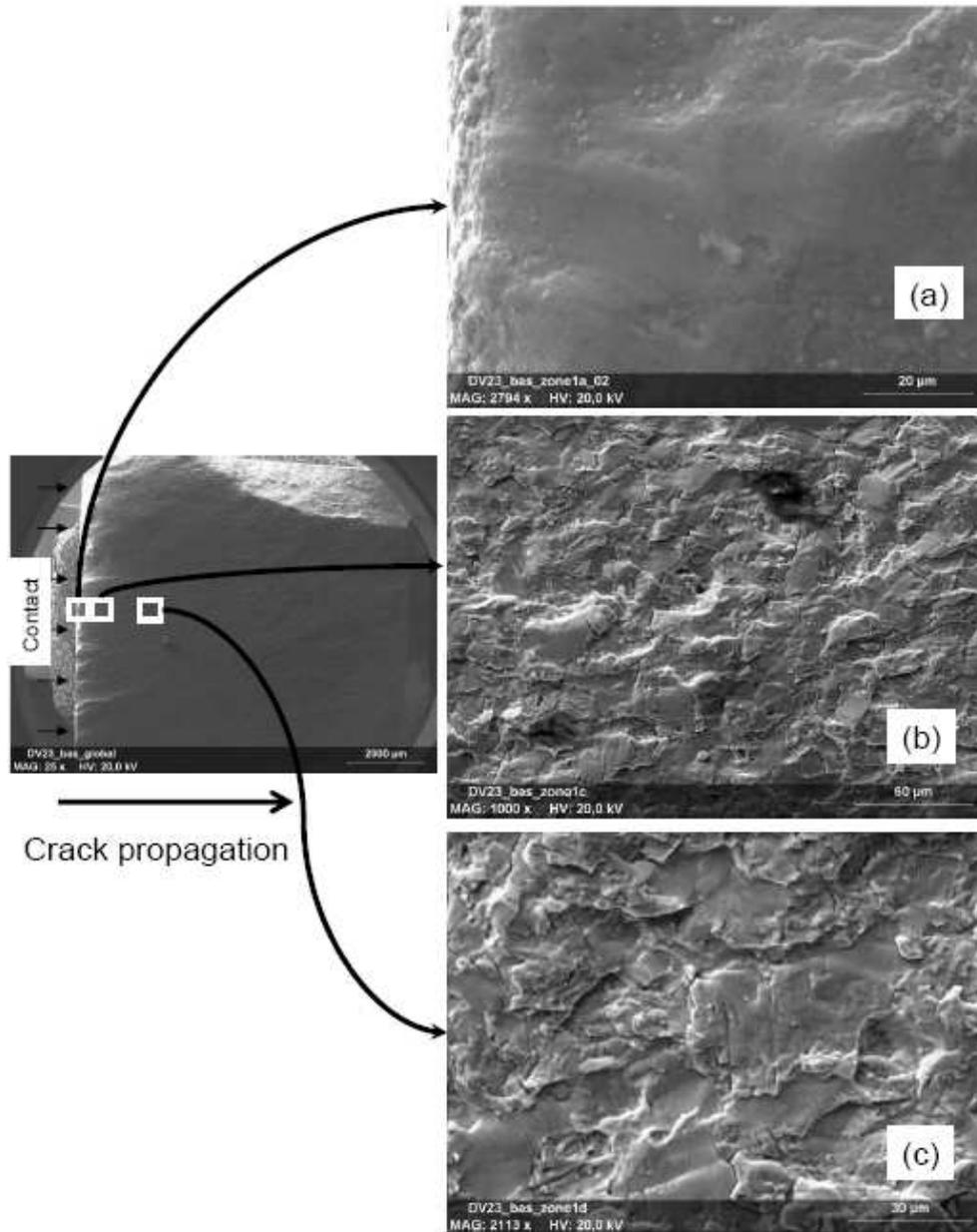
Figure 5: SEM analysis of the fretting fatigue crack growth behaviour for a 'in phase test'
