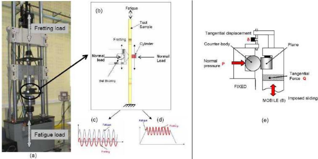
Figure 3: (a) Representation of the LTDS fretting fatigue setup, (b) close-up of the fretting contact and the two types of classical fretting fatigue solicitations: (c) in phase and (d) cyclic constant bulk stress. (e) Schematic of the LTDS fretting system
