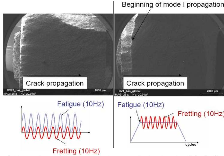
Figure 6: Comparison of fracture faces between the 'in phase' and the 'in flight' tests
