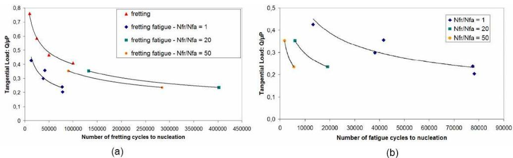
Figure 7: Evolution of the crack nucleation threshold for an  $a_{ref}$  crack in function of the number of (a) fretting cycles and (b) fatigue cycles for each loading combination at 350MPa of fatigue
