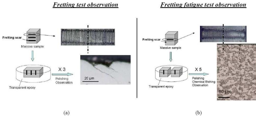
Figure 4: Experimental method to investigate crack length after (a) fretting test and (b) fretting fatigue test
