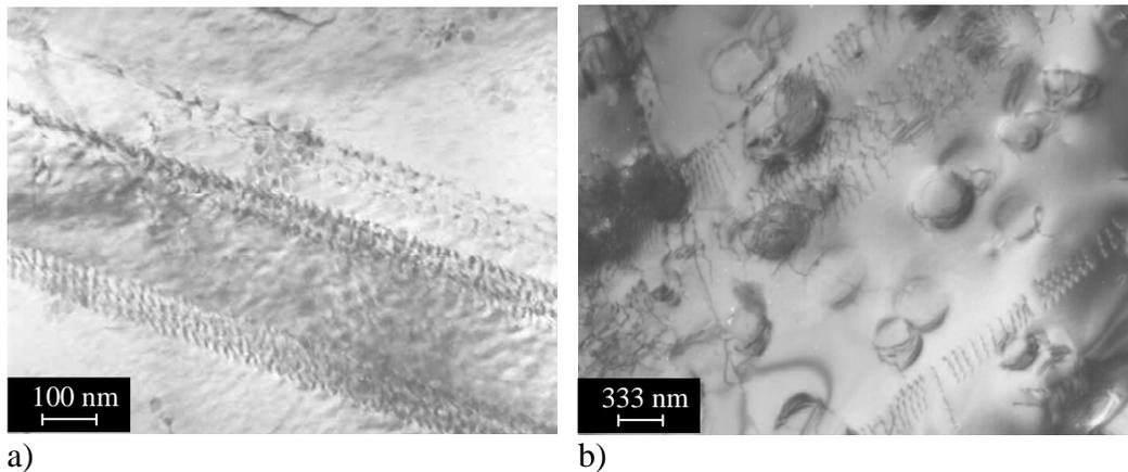
Fig. 4. TEM micrographs comparing the dislocation arrangements in Nimonic 80A after fatigue testing at room temperature in a) the peak-aged and b) the overaged condition.
