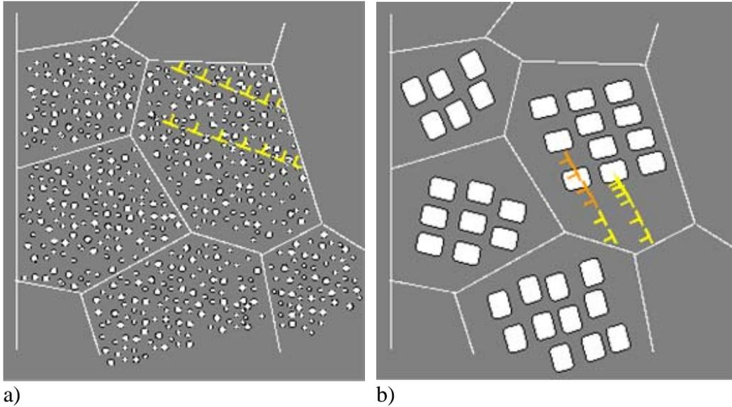
Fig. 6. Illustration of the dislocation particle interaction for the peak-aged and the overaged condition of Nimonic 80A.
