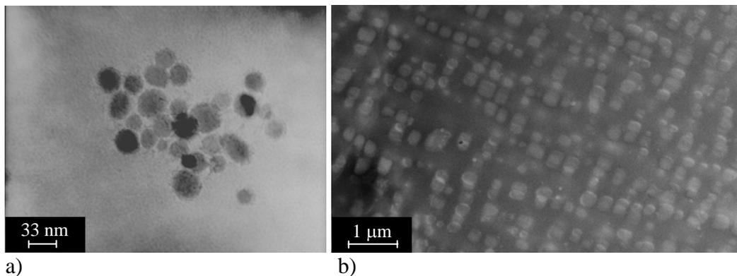
Fig. 1. TEM micrographs of a) peak-aged and b) overaged Nimonic 80A.
