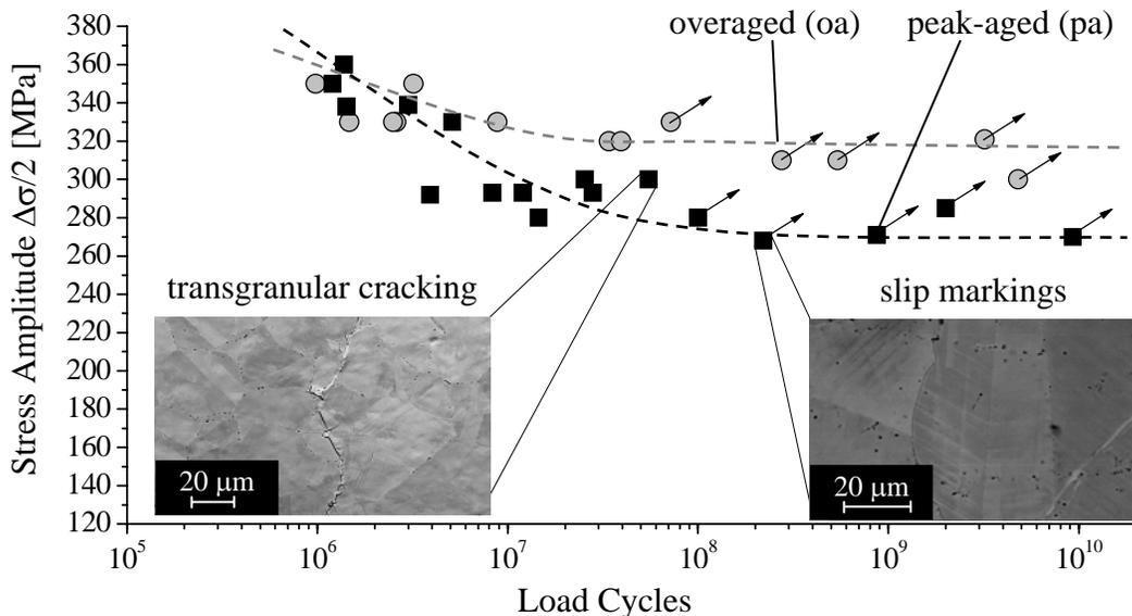
Fig. 2. Fatigue results for peak-aged and overaged Nimonic 80A at room temperature (run-out specimens are marked with arrows).
