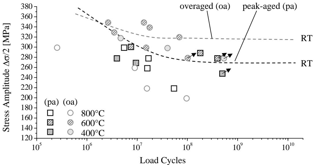
Fig. 3. Fatigue results for peak-aged and overaged Nimonic 80A at elevated temperatures (run-out specimens are marked with arrows).
