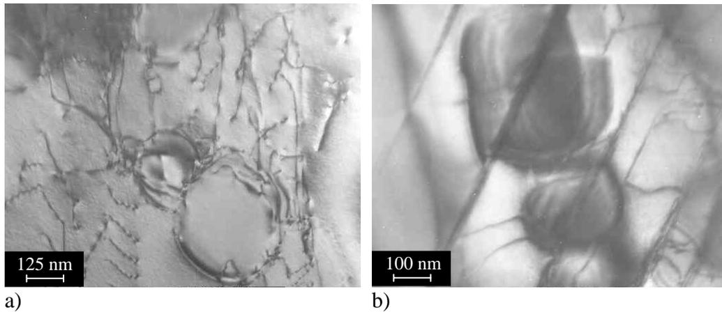
Fig. 5. TEM micrographs of dislocation particle interactions in overaged Nimonic 80A after fatigue testing up to  $N = 1,4 \times 10^7$  at  $600^\circ\text{C}$  showing a) Orowan loops and b) particle shearing.
