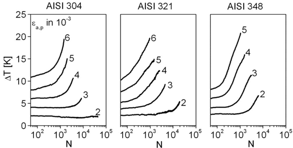
Fig. 5: Development of the change in the temperature  $\Delta T$  as function of number of cycles  $N$
