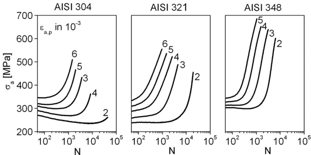
Fig. 4: Development of the stress amplitude  $\sigma_a$  as function of number of cycles  $N$
