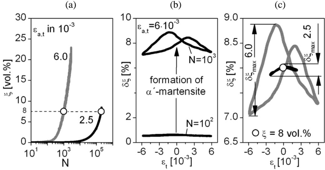
Fig. 7: Development of the  $\alpha'$ -martensite fraction under total strain control (a), magnetic-mechanical hysteresis loops (b) as well as magnetic-mechanical hysteresis loops for a constant  $\alpha'$ -martensite fraction (c) for AISI 321
