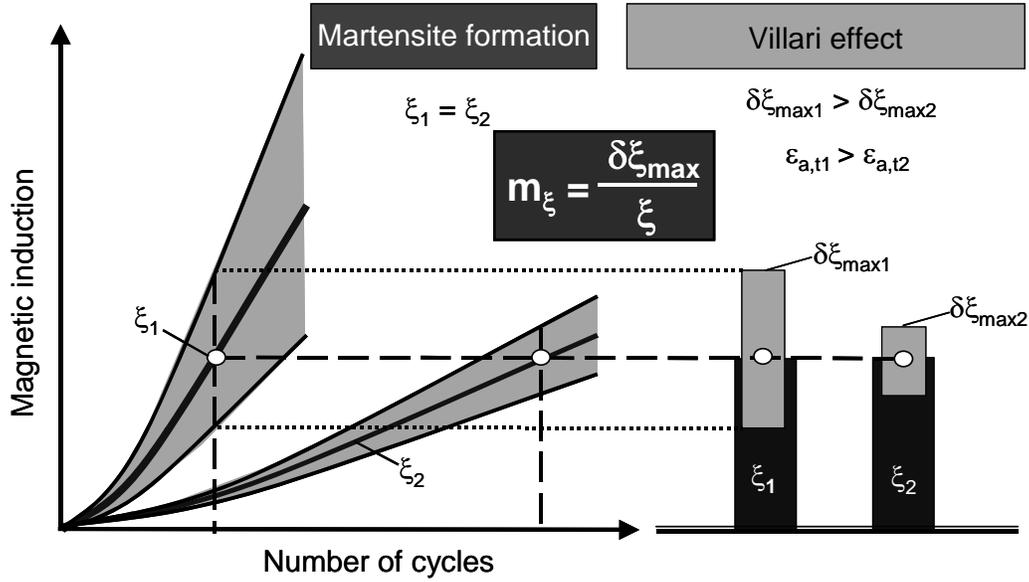
Fig. 8: Fatigue life calculation method for metastable austenitic steels on the basis of magnetic measurements
