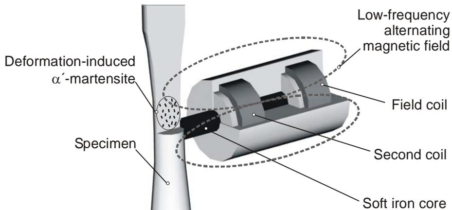
Fig. 3: Measuring principle of ferritescope
