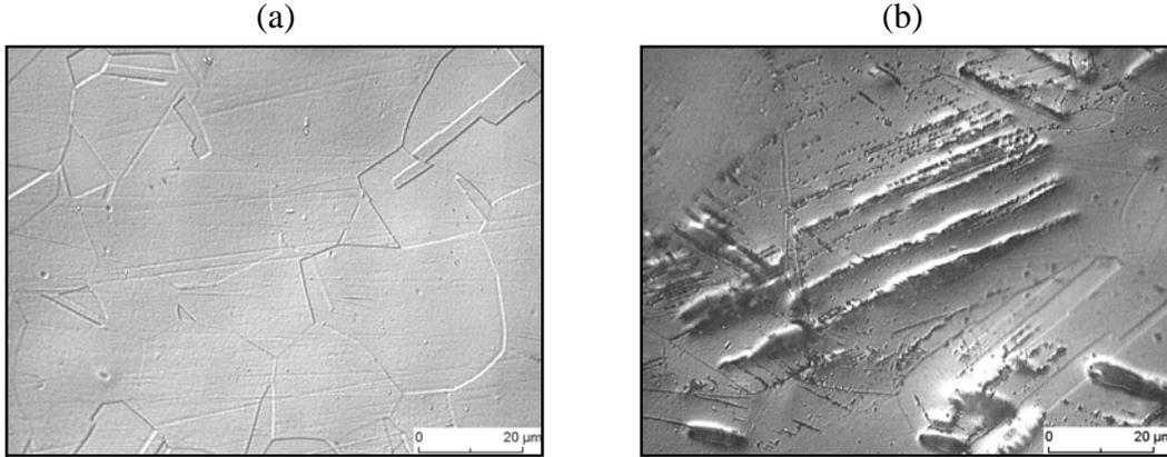
Fig. 1: Optical micrographs of austenite after solution annealing (a) and after plastic deformation with  $\alpha'$ -martensitic needles in an austenitic matrix (b)
