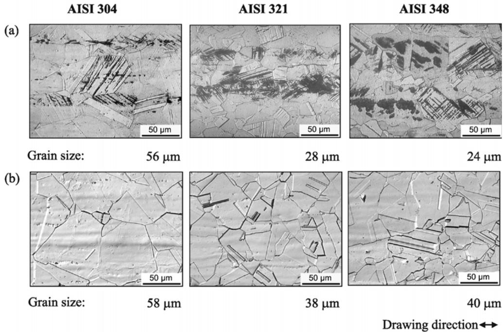
Fig. 2: Optical micrographs in the as-received condition (a) and after solution annealing (b)
