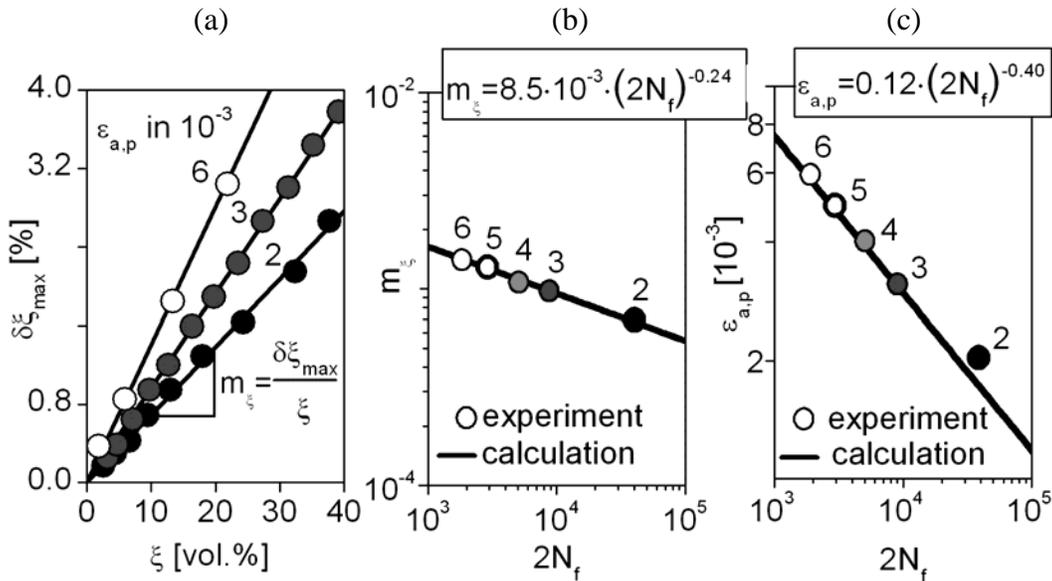
Fig. 9: Maximum change in magnetic induction versus  $\alpha'$ -martensite fraction (a), fatigue life calculation on the basis of magnetic measurements (b) and the plastic strain amplitude (c) for AISI 321
