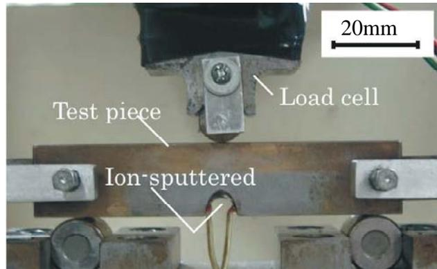
Fig. 5 A view of the test piece with an ion-sputtered film during the test
