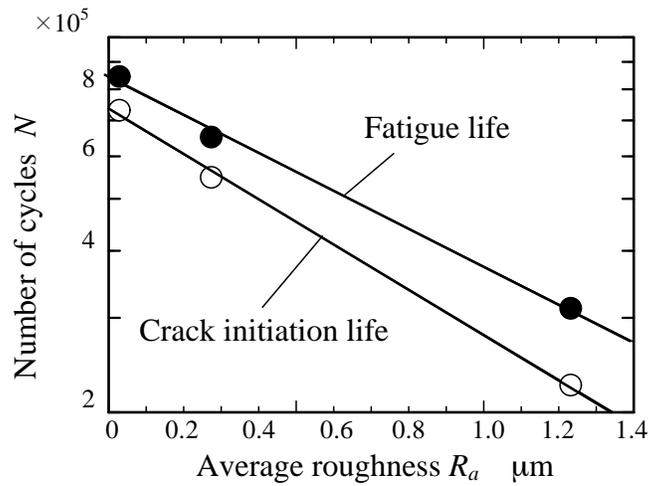
Fig. 9 The fatigue life and crack initiation life vs. the surface roughness
