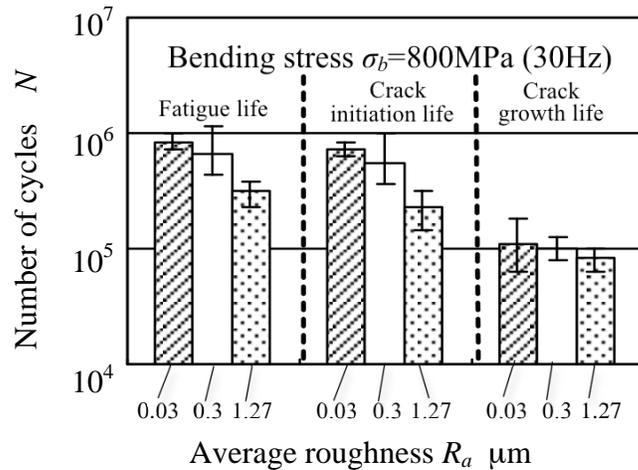
Fig. 8 The fatigue lives of the test pieces in different roughness
