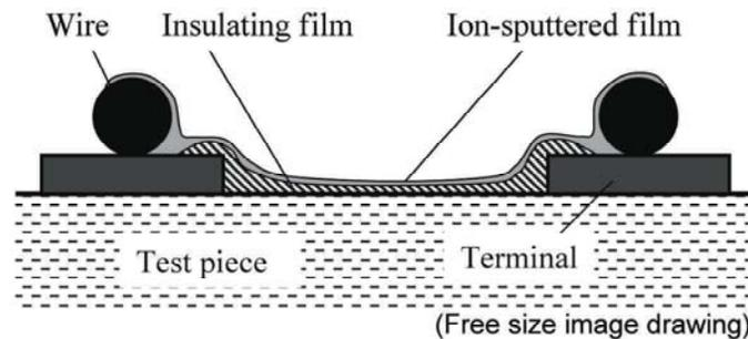
Fig. 4 Section view of the crack initiation detection spot
