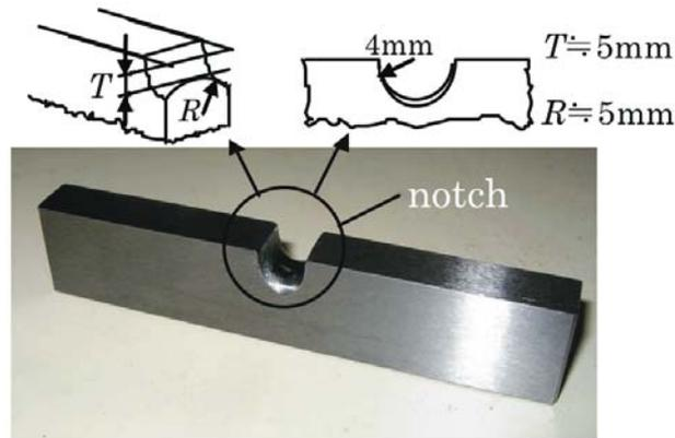
Fig. 2 Test piece with a round notch
