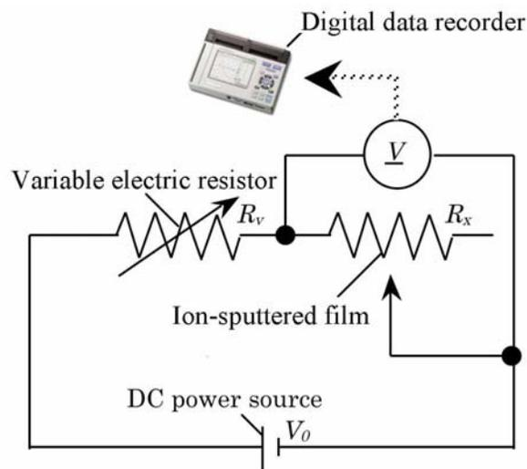
Fig. 6 System used to measure the electric resistance of the film
