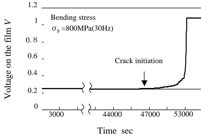
Fig. 7 Electric resistance of the ion-sputtered film during a fatigue test
