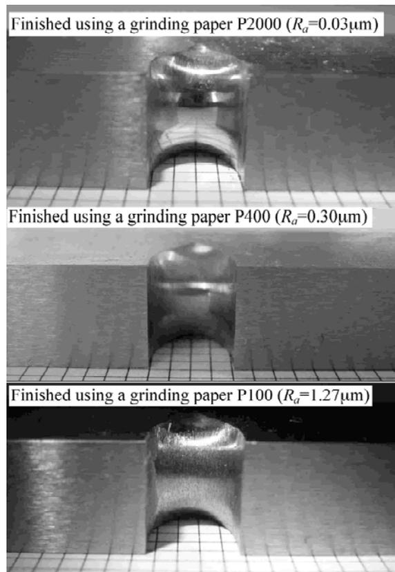
Fig. 3 A view of the three types of notches
