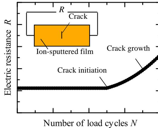
Fig. 1 Change in the electric resistance of an ion-sputtered film due to crack initiation and crack growth
