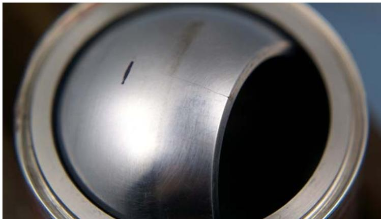
Fig. 2. The partially cracked Ball D
