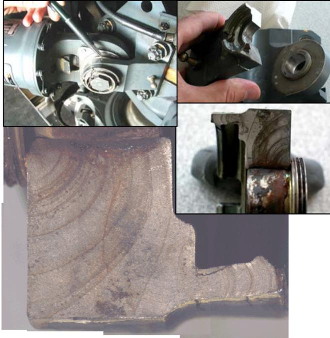
Figure 2 - Metallic Crack Example 1 : SuperPuma MRH damper fitting (Steel)
