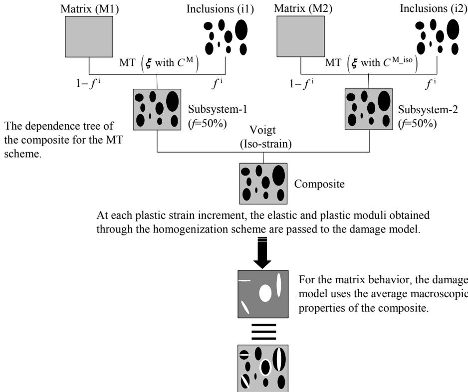
Fig. 1. A schematic diagram showing the dependence tree for the Mori-Tanaka (MT) model and the integration of the MT and the damage models.
