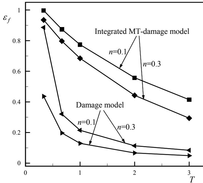
Fig. 3. Variation of the fracture strain  $\varepsilon_f$  as a function the triaxiality ratio  $T$ , for the damage and integrated MT-damage models, for two cases with a different strain hardening exponent,  $n=0.1$  and  $n=0.3$ , respectively.
