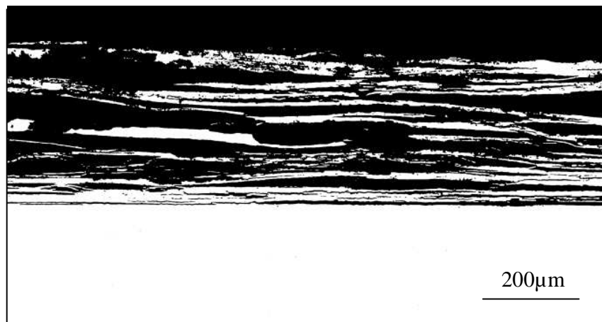
Fig. 1. Exfoliation corrosion as visible on a section of an Al 2024 T351 rolled plate after the immersion test according to ASTM G34.
