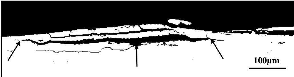
Fig. 4. Intergranular corrosion and first stage of blister formation on the LT-ST cross section exposed during 1 month from the L-LT plane.
