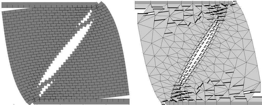
Figure 4: Confined shear wall test with comparison of (left) fine scale modelling results and (right) multiscale modelling results. The same fine scale material parameters were used in both computations.
