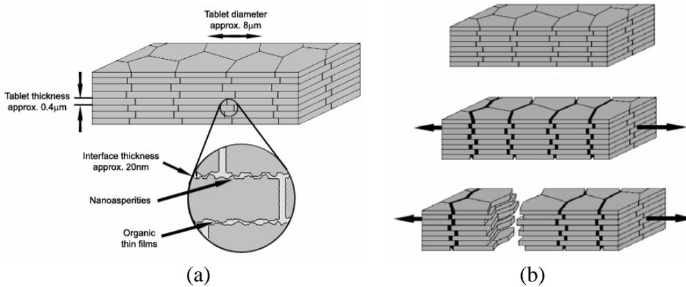
Figure 1: (a) Some key features of the structure of nacre; (b) the prominent deformation mechanism for nacre in tension: tablets sliding on one another.
