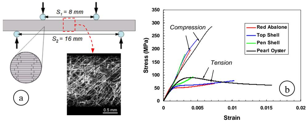
Figure 3: (a) four point bending setup showing microstructure orientation and surface preparation for digital image correlation; (b): Tensile and compressive behavior of four types of nacre
