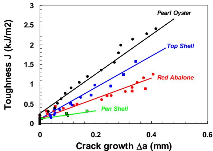
Figure 5: Crack resistance curve for the four types of nacre tested.
