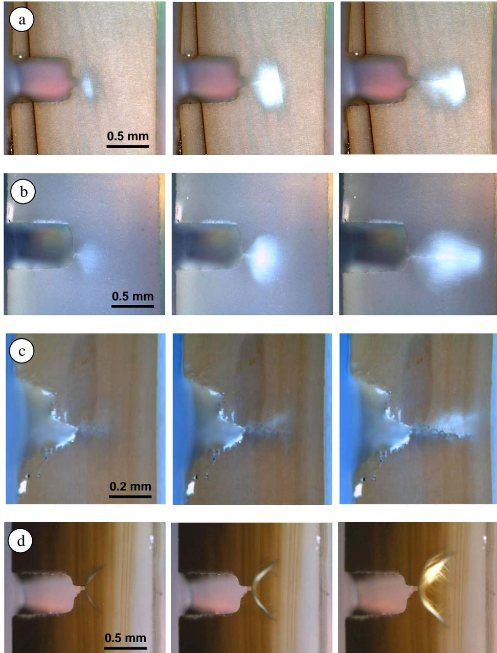
Figure 4: Snapshots taken during fracture tests for (a) Red abalone; (b) Top Shell; (c): Pen Shell; (d) Pearl Oyster.
