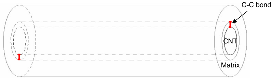
Figure 1: RVE of HAp on tip-functionalized CNT
