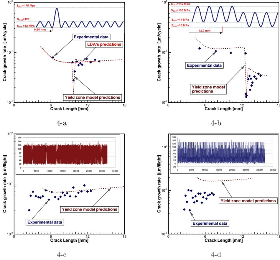
Figure 4: Fatigue crack growth tests results: 4-a. Single overload, 4-b. Block loading (*HI-LO*), 4-c. Flight Spectrum-I, 4-d. Flight Spectrum-II,
