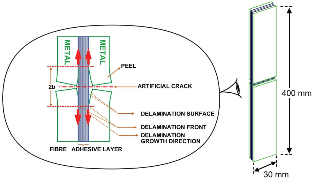
Figure 2: Double cracked lap shear specimen geometry
