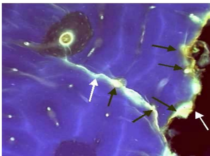
Fig. 2 This illustrates a typical example of two large cracks (white arrows) that were involved in failure of a specimen (the second crack is the main failure surface). As these cracks grew to macrocrack size, they managed to penetrate the cement lines of numerous osteons and used the Haversian canals (black arrows) as weaknesses in which to further propagate.
