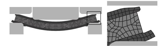
Figure 4: Result of a simulation (left) where the delaminated areas are clearly visible (right).
