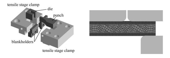
Figure 1: Exploded view of the experimental deep-draw setup.
