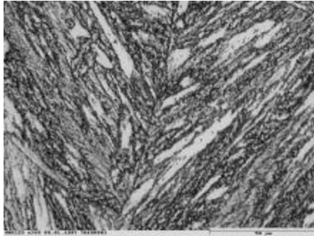
Fig.1 The microstructure of martensitic steel
