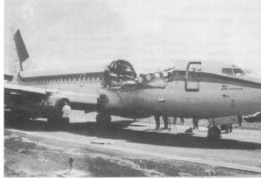
Figure 2. N73711 fuselage failure.
