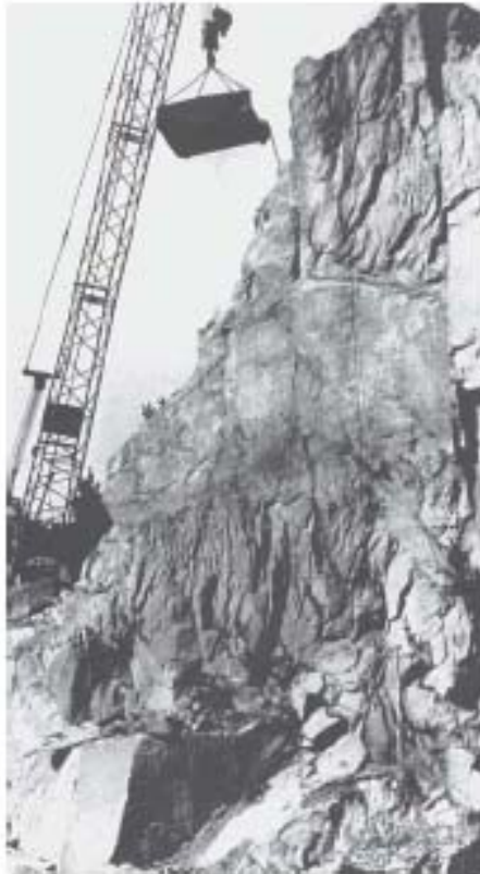
Fig. 7 Joints in the Mrákotín quarry. Photograph of the 025° trending joint A. Vertical ruler is 2 m (from Bahat et al. 2001c)
