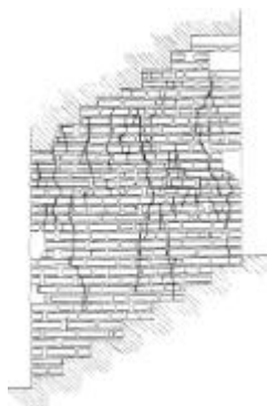
Figure 4: Crack pattern through the thickness of the masonry of the Tower of Monza, corresponding to the opening of a door.
