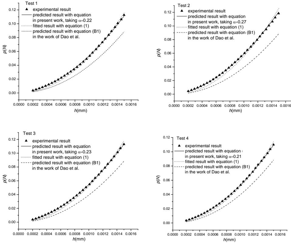
Figure 2: Plot of the experimental  $p - h$  response and corresponding fitted results with the present closed-form expression of indentation loading curves (316 stainless steel)
