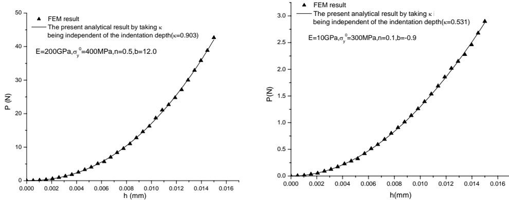
Figure 1: A plot of the present analytical indentation loading curves and the indentation loading curves given by FEM
