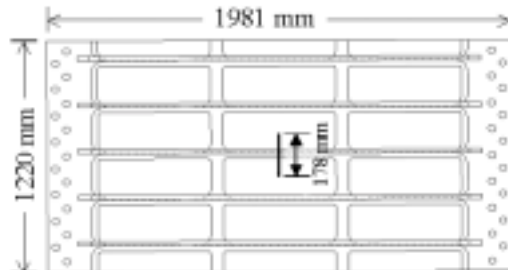
Fig 2. 1220 mm wide curved integrally-stiffened wide panel with a single lead crack.
