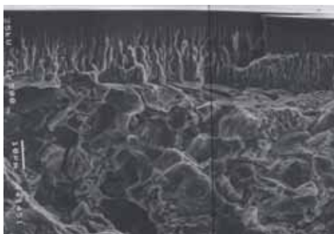
Figure 9: SEM photograph of fracture surface of plated smooth specimen.
