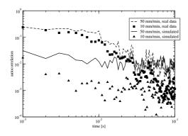
Figure 4: The autocorrelation function of released energy from the in-plane experiment, for two strain rates (10 and 50 mm/min). The data is compared to two artificial timeseries with the same interval and energy statistics.
