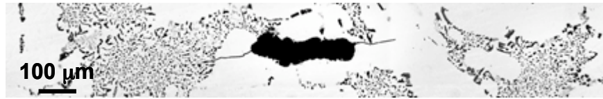
Figure 1: A small crack emanating from a femtosecond pulsed laser notch in W319.
