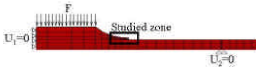
figure 1: Test specimen and boundary condition
