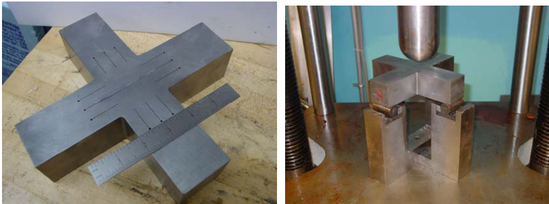
Figure 1 Cruciform specimen and bend apparatus shown without environmental chamber.
