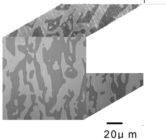
Figure 1: Microstructure for  $\text{Al}_2\text{O}_3/\text{YAG}$  eutectic composite
