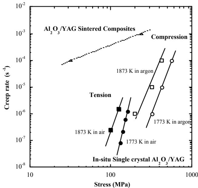
Figure 4: Stress dependence of the tensile creep rate for  $\text{Al}_2\text{O}_3/\text{YAG}$  eutectic composite at 1773 K and 1873 K in air environment, compared with the compressive creep rates for  $\text{Al}_2\text{O}_3/\text{YAG}$  eutectic composite and sintered composite at 1773 K and 1873 K in argon environment
