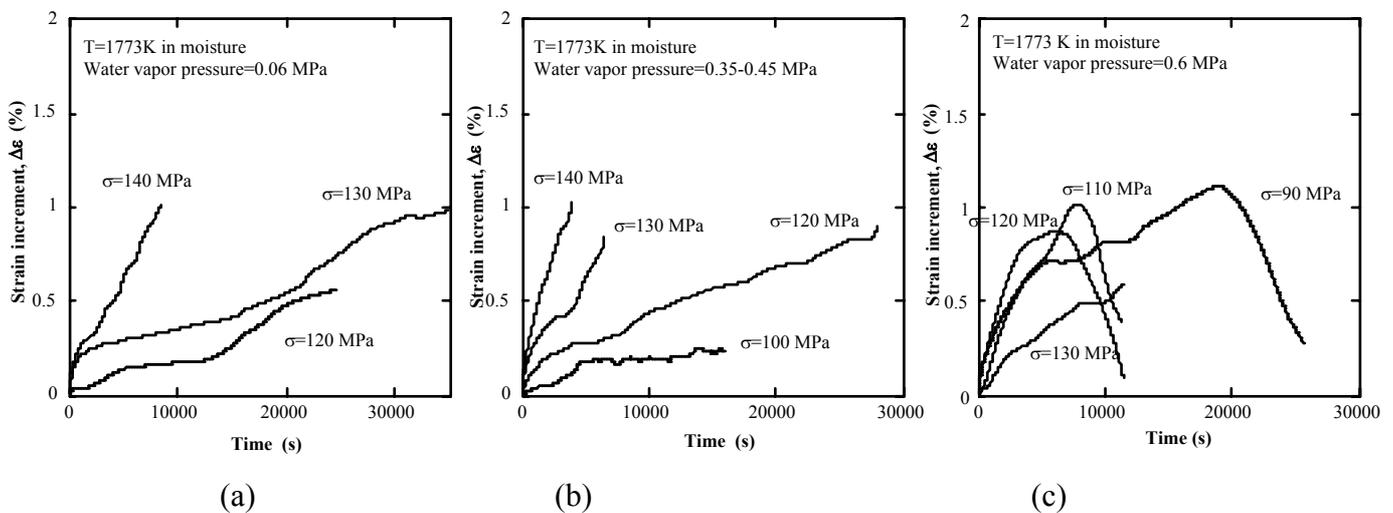
Figure 3: Strain increment as a function of time for  $\text{Al}_2\text{O}_3/\text{YAG}$  eutectic composites at 1773 K in moisture environments, under the water vapor pressure of (a) 0.06 MPa, (b) 0.35-0.45 MPa and (c) 0.6 MPa
