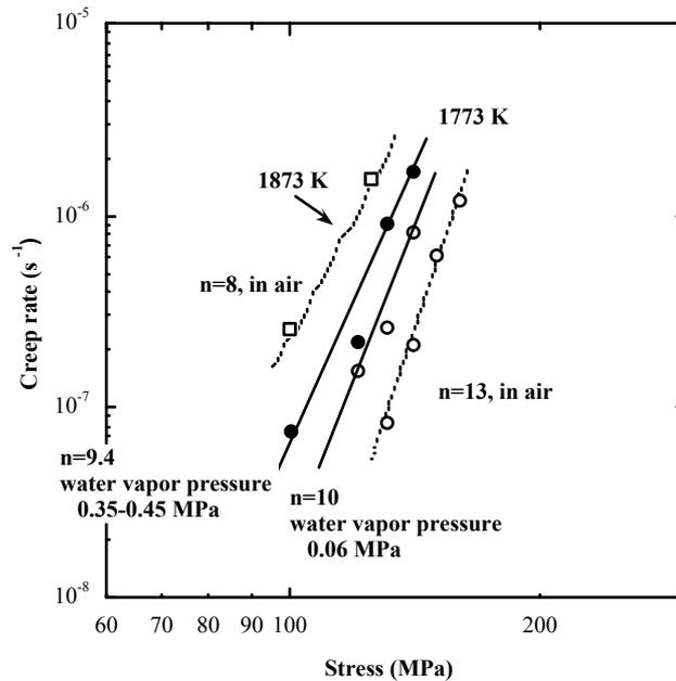
Figure 5: Stress dependence of the tensile creep rate for  $\text{Al}_2\text{O}_3/\text{YAG}$  eutectic composite in air and moisture environments
