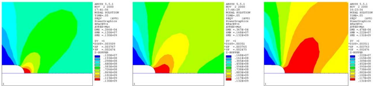
Fig.3 Variation of notch plastic field sizes under different loading levels of maximum stress
