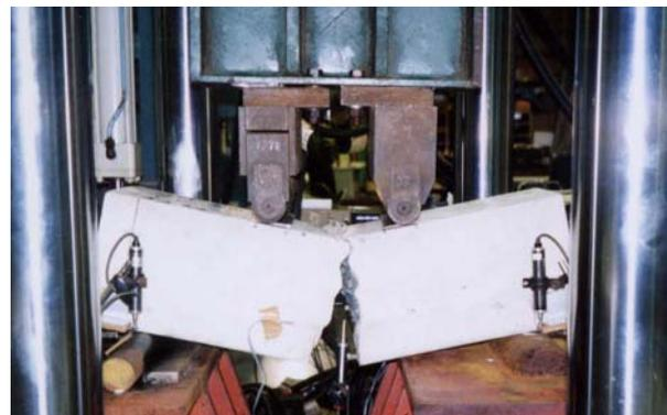
Photo 3: Specimen after failure ( static bend test )
