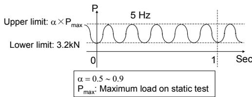
Figure 7: Input condition of load
