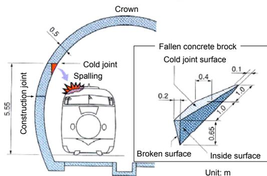
**Figure 3:** Outline of spalling ( illustration )
