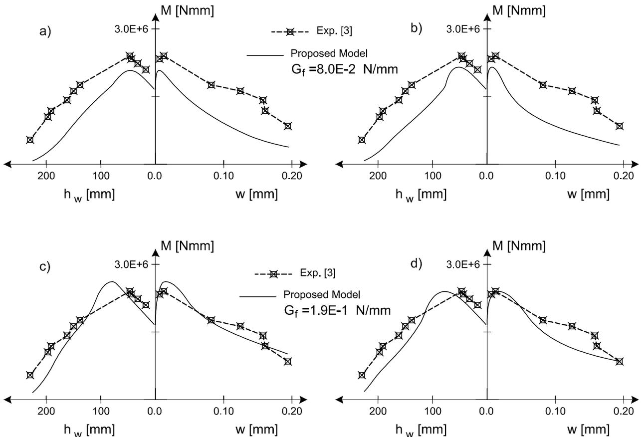
Figure 6: Comparison between experimental and numerical results: a) cohesive bilinear model [16]  $G_f=8.0E-2$  N/mm; b) cohesive exponential model [18]  $G_f=8.0E-2$  N/mm; c) cohesive trilinear model [17]  $G_f=1.9E-1$  N/mm; d) cohesive bilinear model [16]  $G_f=1.9E-1$  N/mm.
