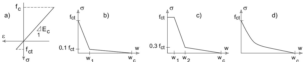
**Figure 4:** Constitutive laws: a) linear elastic law for uncracked concrete; b) cohesive bilinear model [16]; c) cohesive trilinear model [17]; d) cohesive exponential model [18].
