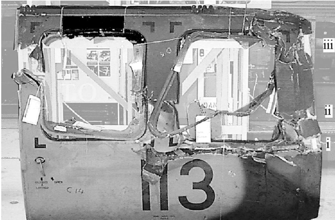
Figure 3 Reconstructed left side cargo door from Black 2 showing three cuts.
