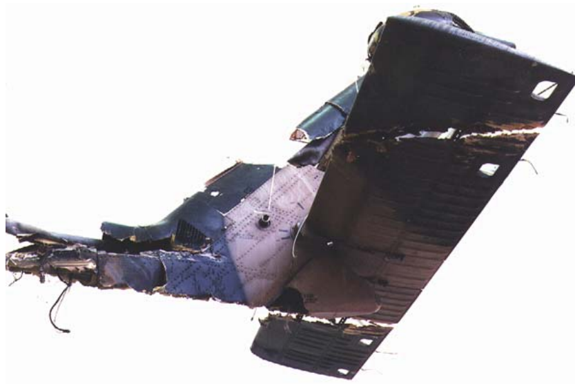
Figure 2 The reconstructed tail section of BLACK 2 looking in-plane with the upper cut through the tail section and the lower cut through the tail boom.
