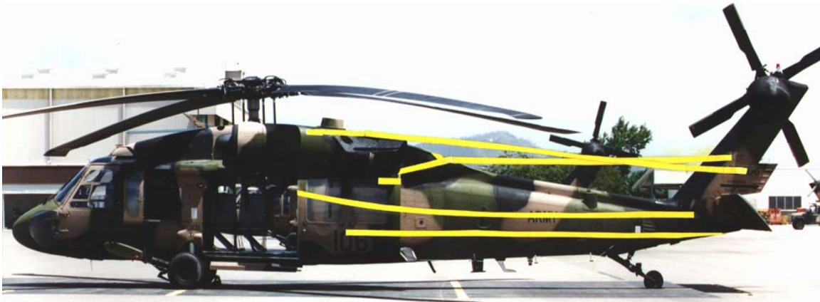
Figure 4 The port side of a Black Hawk showing the deduced positions of the mrb cuts/strikes on BLACK 2
