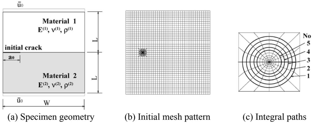
**Figure 3:** Bimaterial plate with an interfacial edge crack
