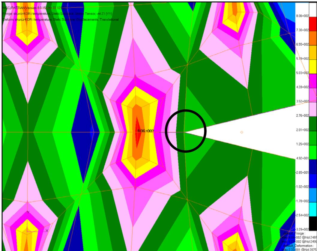
**Figure 3:**  $\sigma_y$  stresses at the crack tip while the load is the same like in the previous case but the phase transformation is simulated in all the grains in the model. The crack tip is constrained to be closed (the scale for displacements: 30:1).
