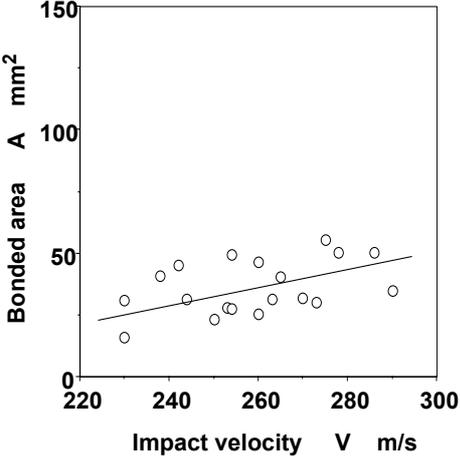
Fig. 4 Effect of impact velocity on bonded area
