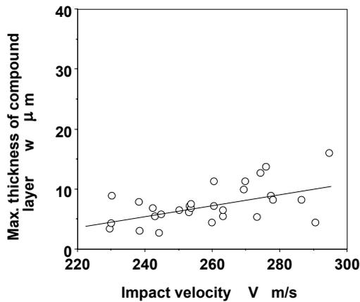
Fig. 6 Maximum thickness of compound layer plotted against impact velocity
