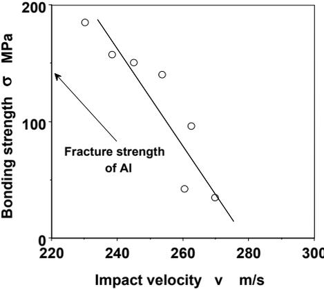
Fig. 8 Effect of impact velocity on bonding strength
