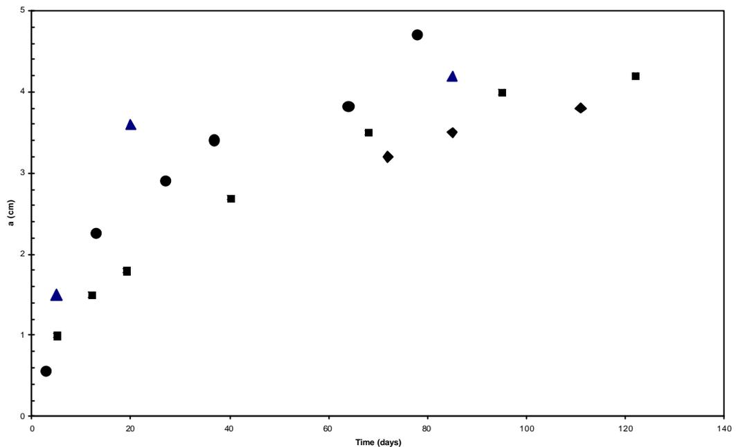
Figure 7. Measured crack lengths at different external stresses.
