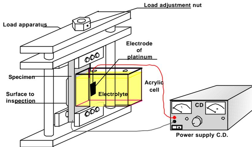
Figure 1. Loading frame and cathodic charging set up.
