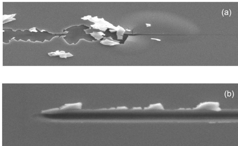
**Figure 1:** SEM micrographs of scratch tracks for (a) sample with interface delamination ( PVD, 4.2 monolayers of silver), and (b) sample without interface delamination ( PVD,  $<0.8$  monolayers of silver).
