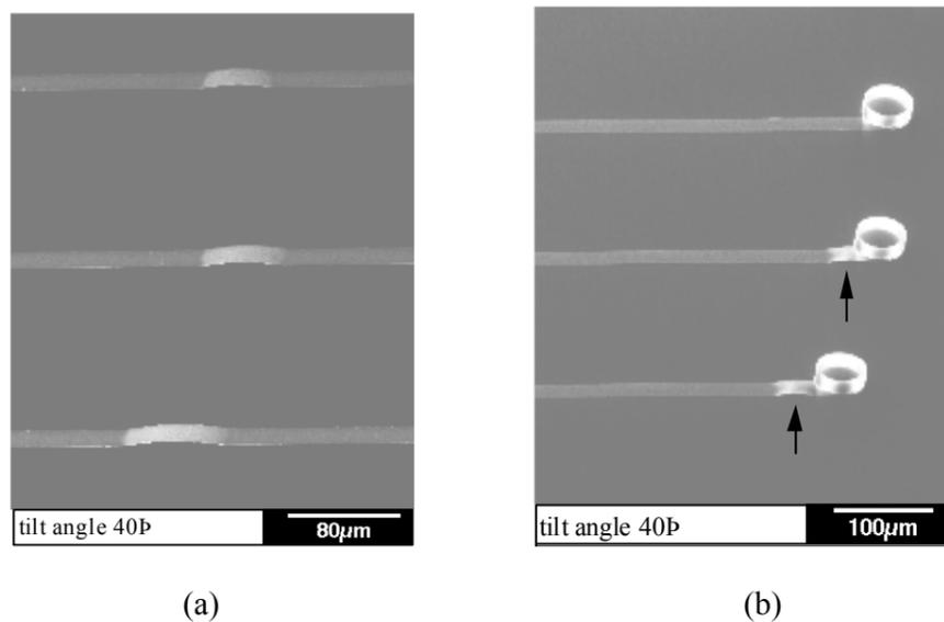
**Figure 4:** SEM pictures of (a) buckled niobium lines on sapphire substrate (PVD, 3.0 monolayers of silver), and (b) curled photoresist/niobium bilayer lines on a sapphire substrate with lines detached from the substrate at the niobium/sapphire interface (PVD, 2.1 monolayers of silver). The arrows point to buckles.
