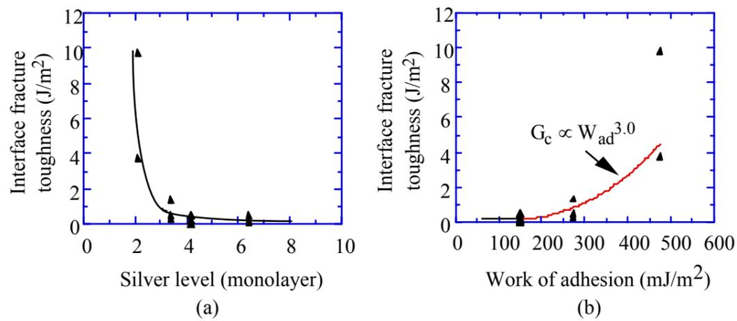
**Figure 2:** Interface fracture toughness of niobium/sapphire interface as a function of (a) silver level at the interface, and (b) work of adhesion of the interface, and a least squares power law fit yielding  $n = 3.0$ .
