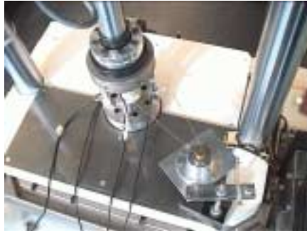
Figure 1: Set-up for measurements of the rotational angle
