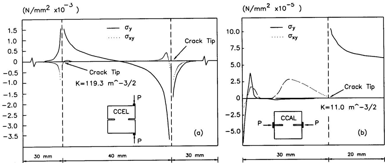
Figure 1. Distribution of  $\sigma_y$  and  $\sigma_{xy}$  along the crack plane
