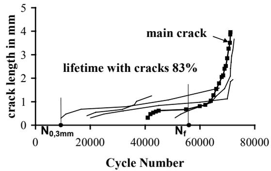
b) Typical crack initiation and propagation
