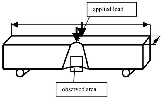
Figure 1. 3-point bending specimens
