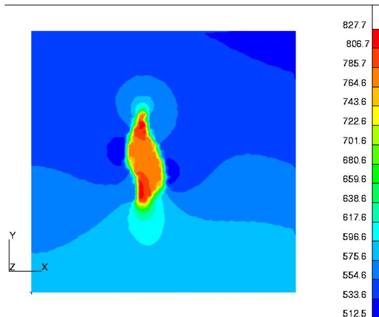
Figure 4. Von Mises stress distribution in the real microstructure of the steel in the notch of the specimen.
