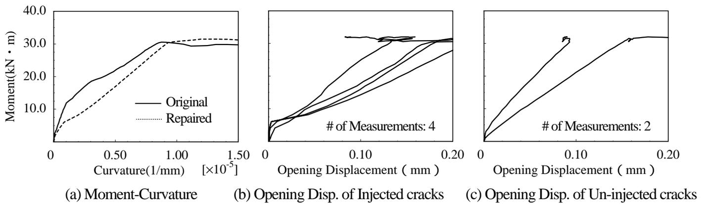
**Figure 6:** Mechanical Properties of Repaired Reinforced Concrete Beams with Polymer Cement Slurry Injection
