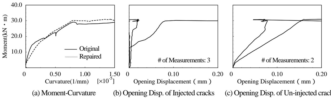
**Figure 5:** Mechanical Properties of Repaired Reinforced Concrete Beams with Epoxy Injection
