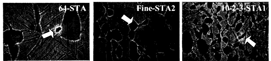
Fig.4 Micrographs of longitudinal sections of smooth specimens.
